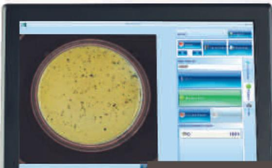
Once a plate is inserted, the locating pins centre the sample. Assays are treated in batches which are defined before counting or measuring. Designing a batch includes assay type, colour, size and shape classification. After the 'measure' button is touched to activate counting, colonies are immediately detected and the count is displayed on screen.
