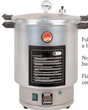
Auto-Koch produced by International Pbi is a 23 litres transportable steam steriliser for laboratory and medical use as an aid to R & D.
